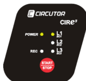
Fig. 6-22.- Wrong connection indication (L2 and L3 blinking)
