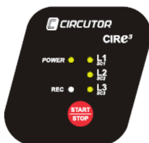
Fig. 6-26.- Indication of proper connection (all LED permanently lighting)
