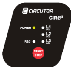
Fig. 6-18.- LED indicators showing the status of CIR-e 3
